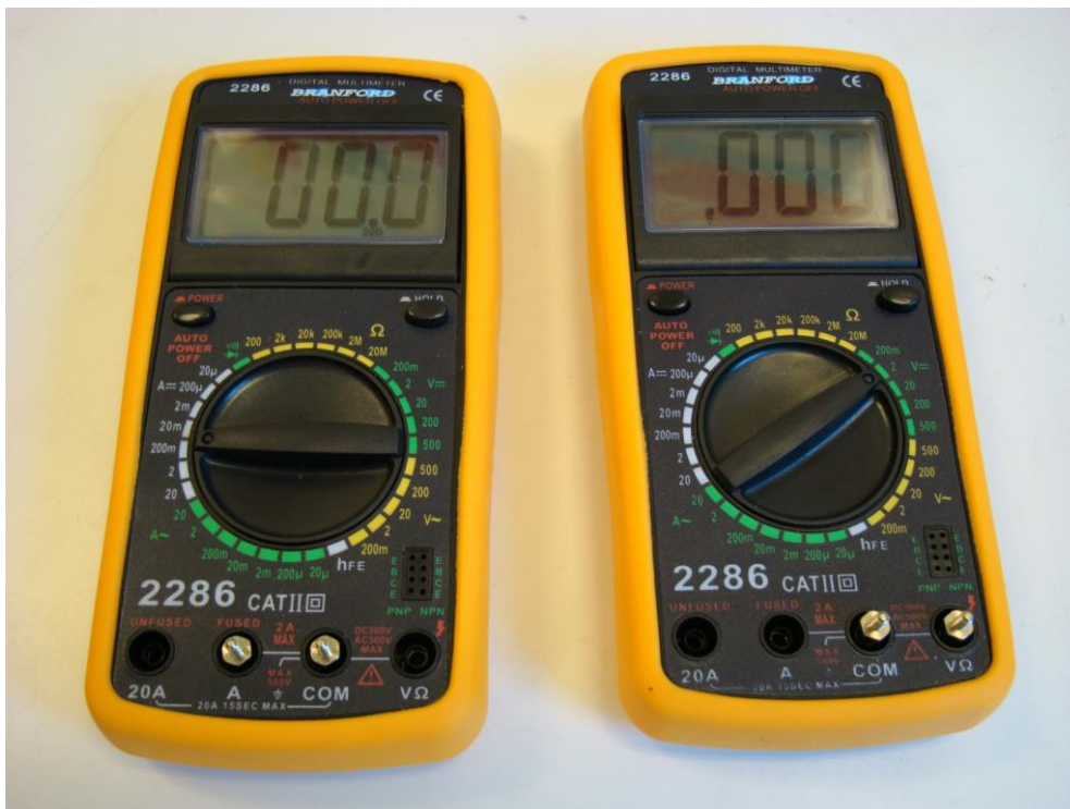
Figure 2.3 Multimeters equipped with terminals for use as ammeter (left) and voltmeter (right), respectively. The instrument is turned on by pressing “POWER” in the top left corner. The instrument turns off automatically after a certain idle time. It can measure direct current and voltage (=) as well as alternating current and voltage (~). The internal resistance in the voltmeter is 10 M \Omega regardless of the measuring range. The potential difference over the ammeter is 200 mV at full reading, regardless of the measuring range. In case of overflow the display will show “1”, and you need to select a higher measuring range. The “HOLD” button (top right corner) should not be pushed, except if you want to freeze a measurement.
