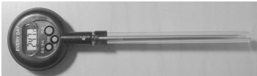
Photo IV-5. Thermometer: The thermometer shows Celsius reading. If Fahrenheit reading is shown, ask Lab Assistance. Read the temperature only, do not touch.
