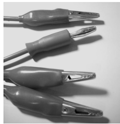
Photo IV-4. Connecting wires. Two types of wires are provided: alligator- alligator and alligator-banana.
