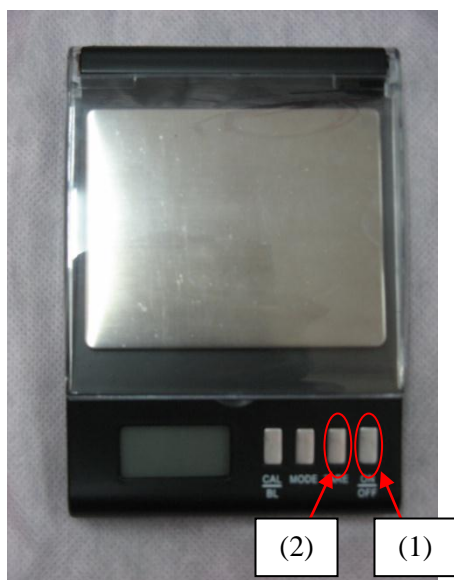
Figure 2: The digital scale (1) On/Off button (2) "Tare" button – sets the current weight as 0.
